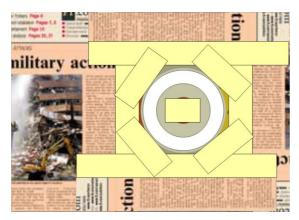
Mask up being careful to protect all the exposed areas including the alignment marks, stencil label, and the orientation arrow.
